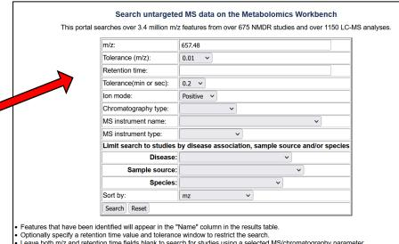
Leave both m/z and retention time fields blank to search for studies using a selected MS/chromatography parameter.
